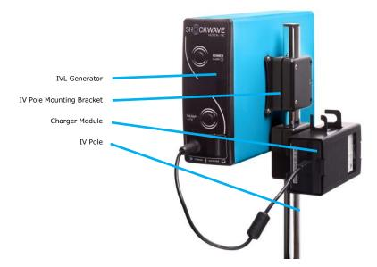
Care should be taken in selecting a stable pole that has a wide base and locking-style casters. An IV pole with five casters, located in a circular pattern with a diameter of at least 19 inches (48.26 cm), such as the Shockwave IVL Stand (or equivalent) is recommended.
